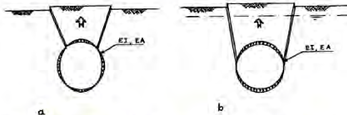
Figure 4. Soil failure for a shallow tunnel; a) breaking up of the tunnel roof due to vertical ovalisation. b) Buoyancy of a shallow tunnel with high groundwater level.
